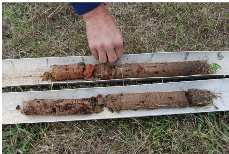
Figure 4 800mm cores from the garden site illustrating broken rock fragments from fill material
