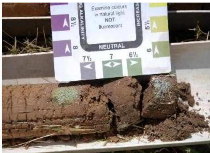
Figure 15 Field pH test (~ 6) on soil core from proposed garden area
