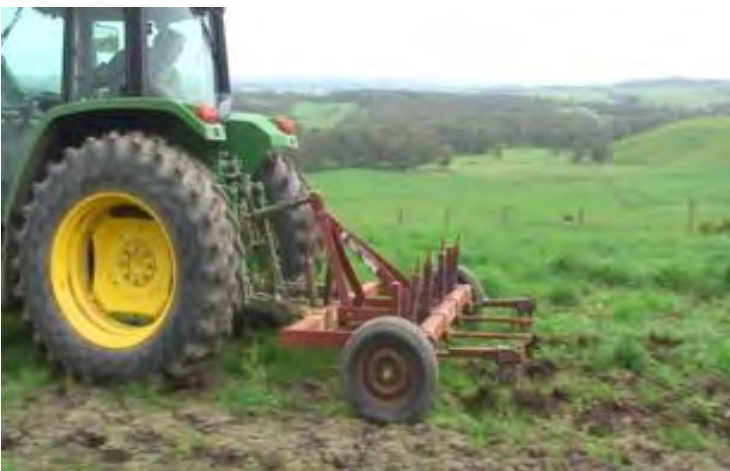
Joe with the agro-plough set up as a 4 tined aerator
