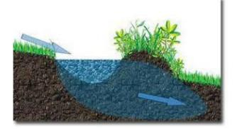
swale below the mound and beyond, where it is effectively stored in the ground away from evaporation where it is needed, rather than simply running down the catchment and disappearing, or evaporating in a dam.
